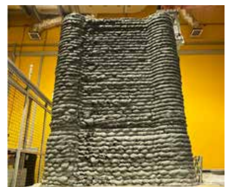
Figure 7: Aramco 3D Concrete Printing with large aggregates and CO 2 curing
