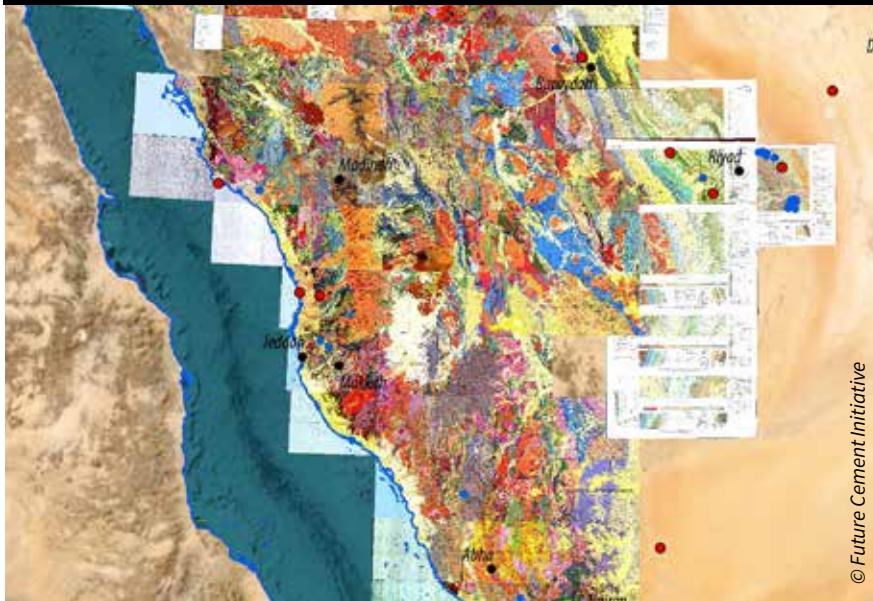
Figure 2: Geological maps (1:250,000) by the Saudi Geological Survey. Red dots represent cement plants and blue dots are location of surveyed sites
